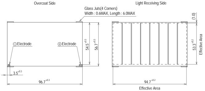
Note: Glass Substrate Thickness : 1.1mm Module Thickness : 1.3mm max Accepts normal soldering for bending.
